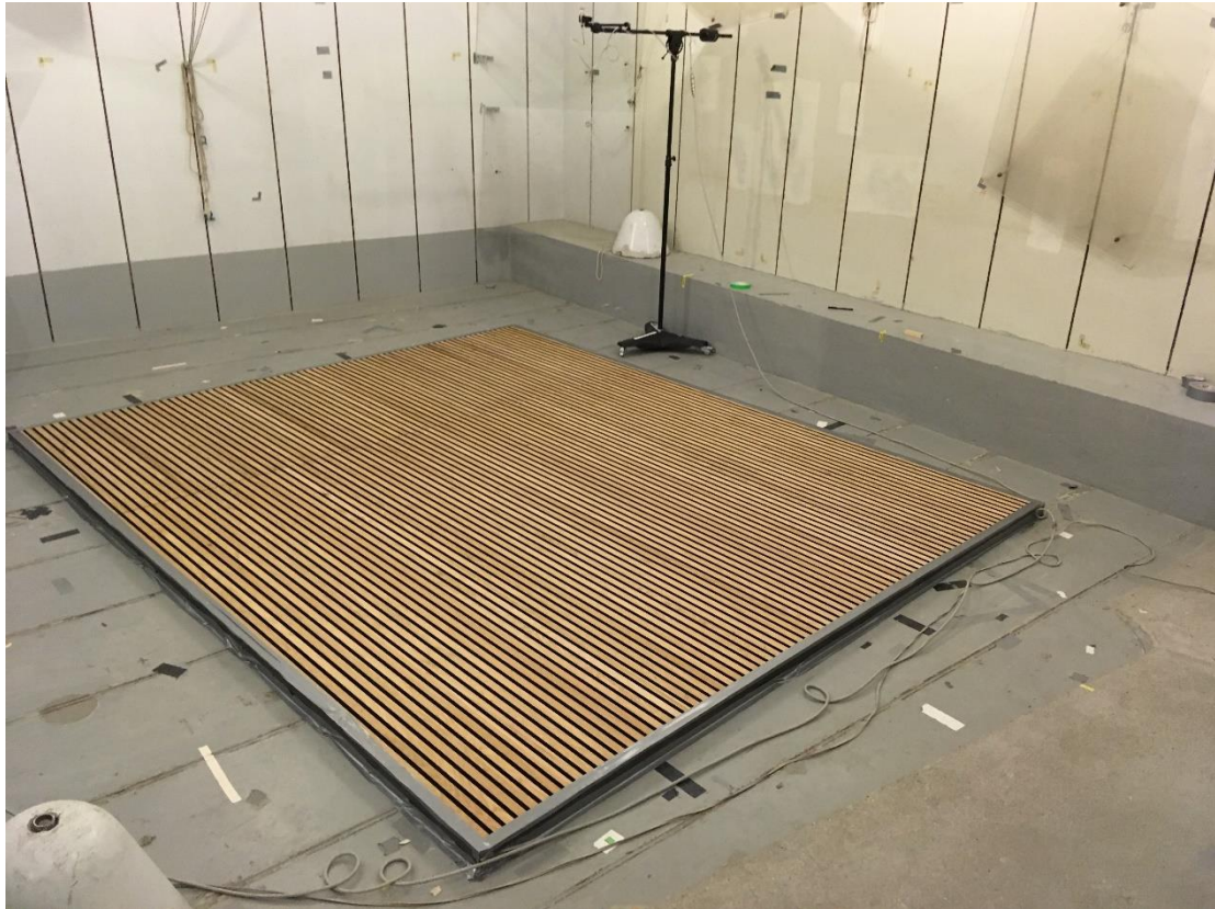
WoodUpp Akupanel mounted in the laboratory.
